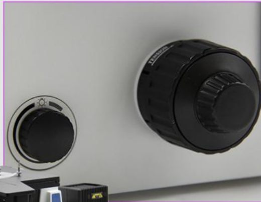
Coaxial Coarse & Fine Focusing System With Adjustable Tension, Coarse Range 9mm (6.5mm up & 2.5mm down), Fine Precision 2 \mu m
