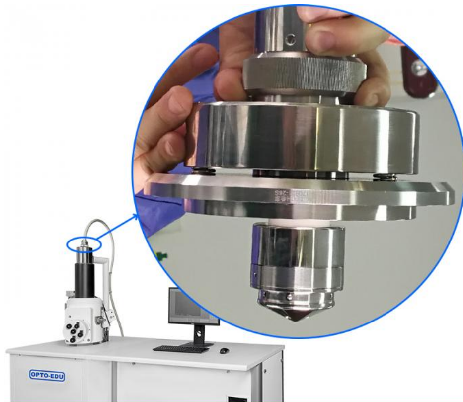
Pre-Centered Tungsten Filament Cartridge Electron Gun Electron Gun Room Vacuum > 2.6 \times 10^{-3} \text{ Pa}
