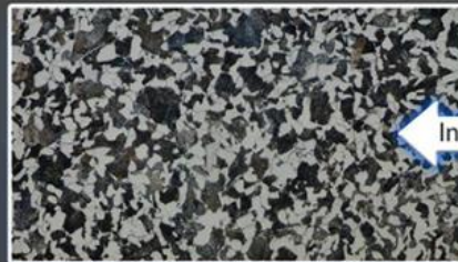
Carbon Steel (Objective: 50X)
