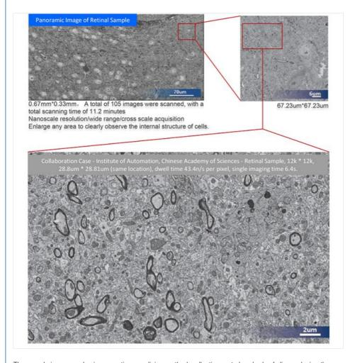
The sample is prepared using a continuous slicing method, collecting up to hundreds of slices, placing them on a sample circle, and loading them into SEM at once.
