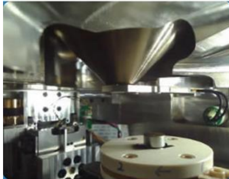
Addition of a camera inside the sample compartment for real-time observation of the sample compartment
