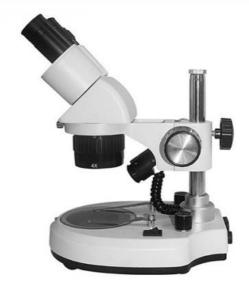
WF10x Eyepiece 1 Pair, With Objective Reach Magnification 10x-40x Binocular Head Inclined 45° Interpupillary Distance Adjustable
