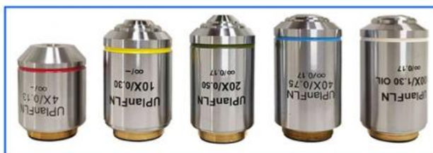
A5F.2611 Infinity Plan Semi-APO Fluorescent Objective
