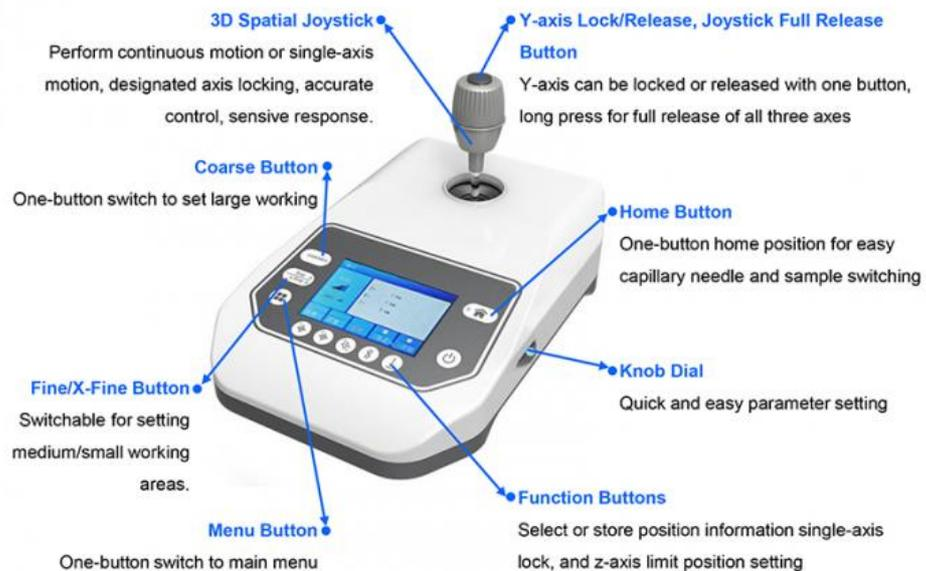
Move smoothly without jitter or delay in the X, Y, Z three-dimensional.
