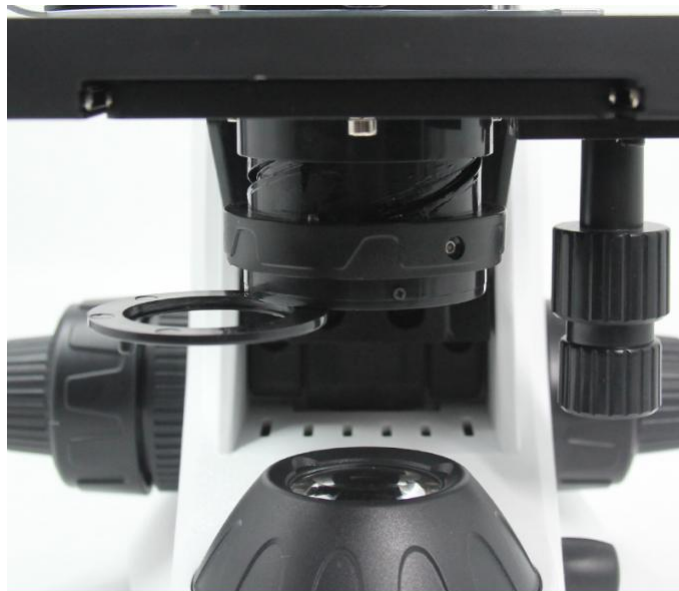
Abbe Condenser N.A.1.25, Iris Diaphragm, Spiral Up/Down 3W LED Illumination With Aspheric Collector
