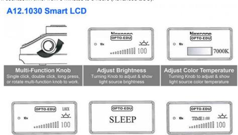
Sleep Mode ick knob to switch betwo Working Mode quickly. Auto Power Off Timer Long press knob for 3s to set 8 show auto power off timer
