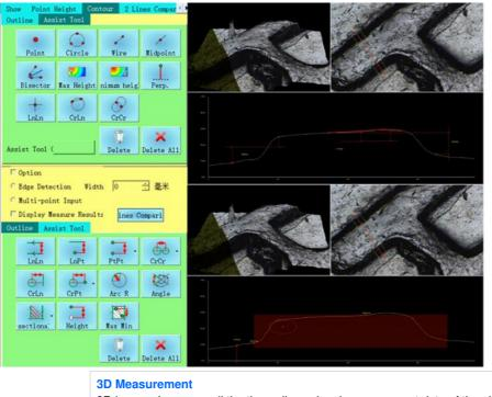
3D image also saves all the three-dimensional measurement data of the observed object, and supports any measurement of the observed object later, including the height, depth, length, roughness, convex area, concave area, convex volume, concave volume, etc
