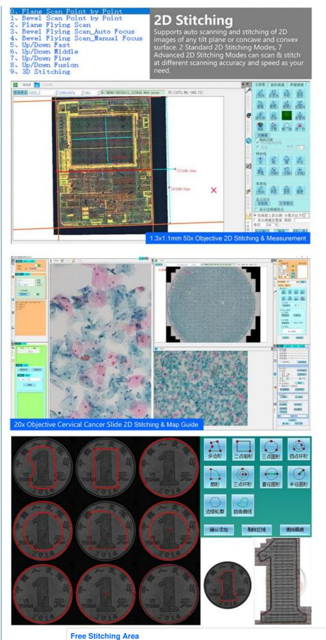
10 stitching area modes can quickly set stitching areas of any shape. Outline mode can automatically detect the edge contour of the object as the stitching area.
