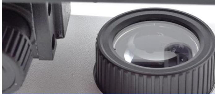
6V20W Halogen Lamp With Brightness Control
