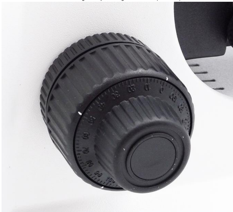
Coaxial Coarse & Fine Focusing
