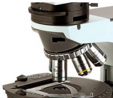
Polarizing Rotatable Stage, Center Adjustable Minimum Reading 6' By Means of Vernal Scale 45° Click Stop Knob
