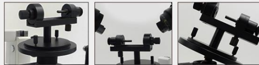
○ Bullet Holder Set To Hold & View All Kinds Of Cartridge, Bullet, Other Objects In Different Angle And Position Freely. Each Microscope Include 2 Sets
