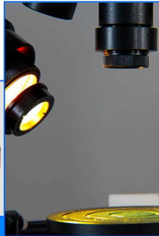
Coaxial Light Attachment to get vertical light path for watching inside deep hole bottom
