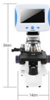
Coaxial coarse & fine focusing, to focus the image clear easily
