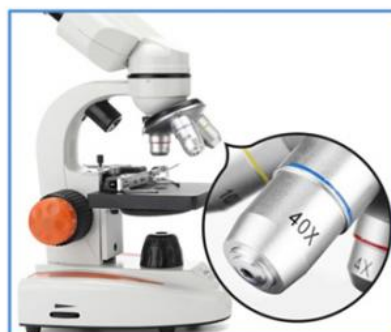
Backward triple revolving nosepiece, Achromatic 4x, 10x, 40x
