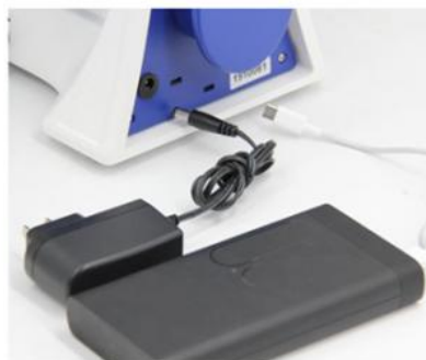
Low Voltage Power Supply By External 5V Adapter, Or USB Power Bank
