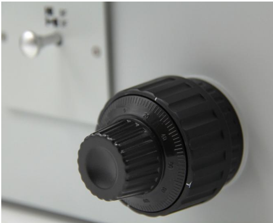
Coaxial Coarse & Fine Focusing System With Adjustable Tension, Coarse Range 9mm (6.5mm up & 2.5mm down), Fine Precision 2 \mu m
