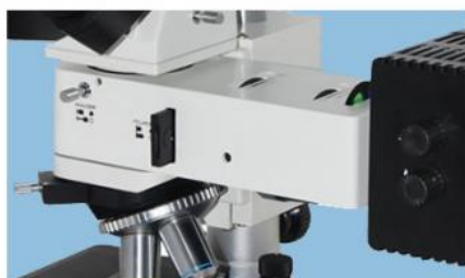
Epi-Illumination 6V30W or 12V50W, Integrated With Field Diaphragm, Aperture Diaphragm, Y/G/B Filter Switch Disc, Push-Pull Polarizing Device
