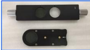
A5P.2603-BKR Analyzer + Polarizer For Reflect Light
