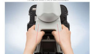
To Hold The Microscope in Comfortable Steady Position
