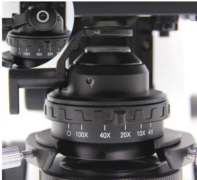
Swing-out Condenser,N.A.0.9/0.13,Iris Diaphragm
