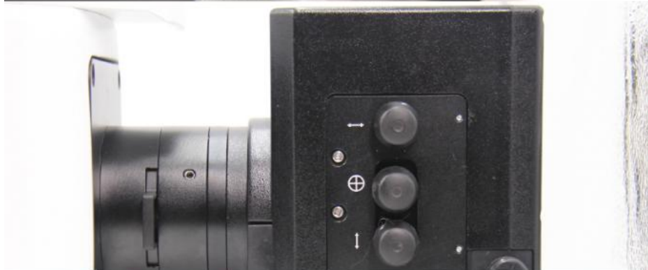
High Brightness Reflect Light Halogen 12V50W Koehler Illumination
