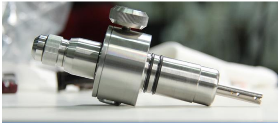
3 Molybdenum Objective Apertures, Adjustable Outside Of Vacuum System, No Need Disassemble Objective To Change Aperture
