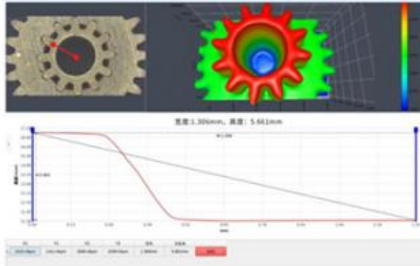
Stereo Microscope Watch Gear Height 5.661mm
