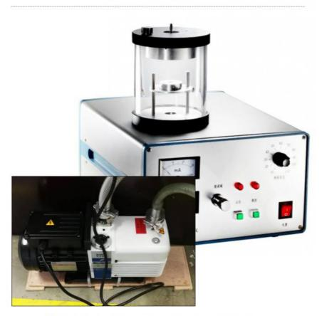
O The Pump Used To Make Low Vaccum For Ion Sputtering Coater
