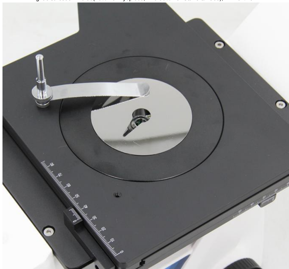
Three-layer Working Stage, Stage size: 180 × 155mm
