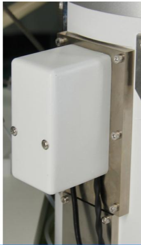
SE: High Vacuum Secondary Electron Detector (With Detector Protection)
