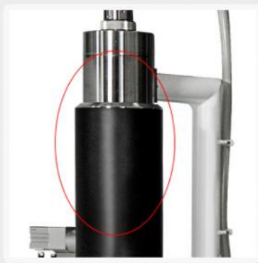
○ The Electromagnetic Lens In This Cylinder
